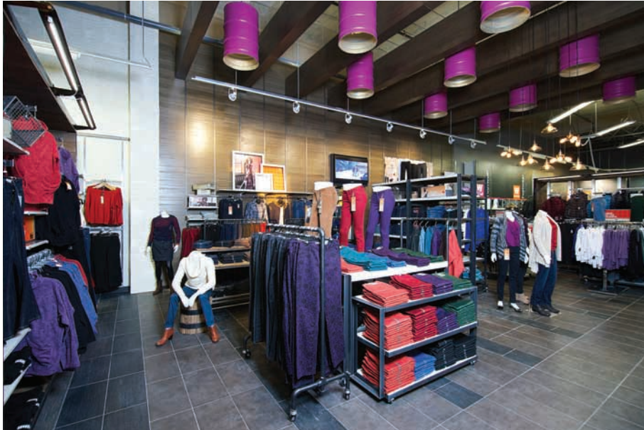
Industrial touches in the womenswear department are softer and more playful. Wood in the display fixtures has a whitewashed finish, walls finished in brick veneer and painted off-white add character, while light fixtures made of oil drums painted fuchsia hang between wooden beams replicating the look of an old factory ceiling.
